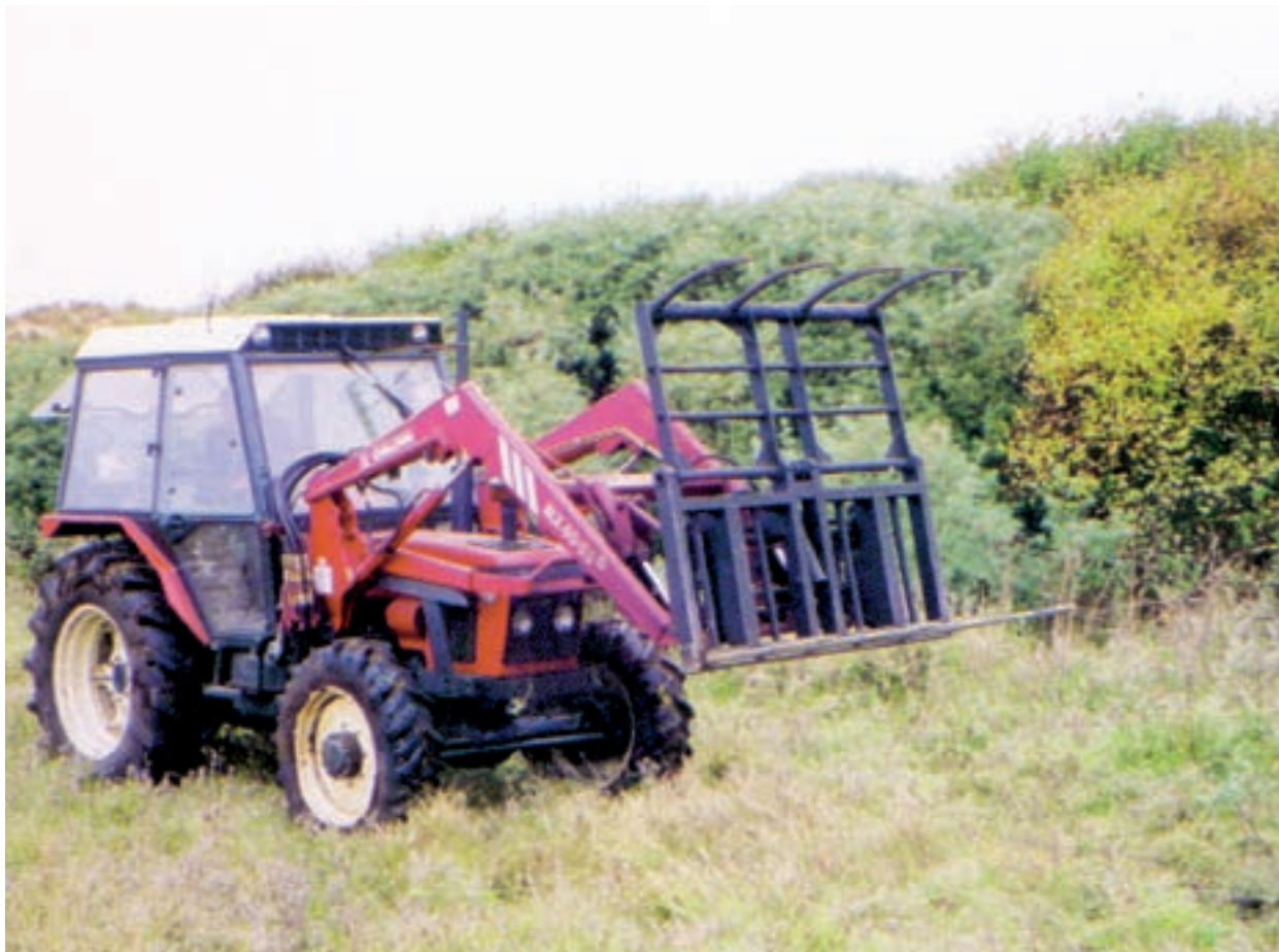
Plate 7 Wide-gape grab on four-wheel drive tractor.
