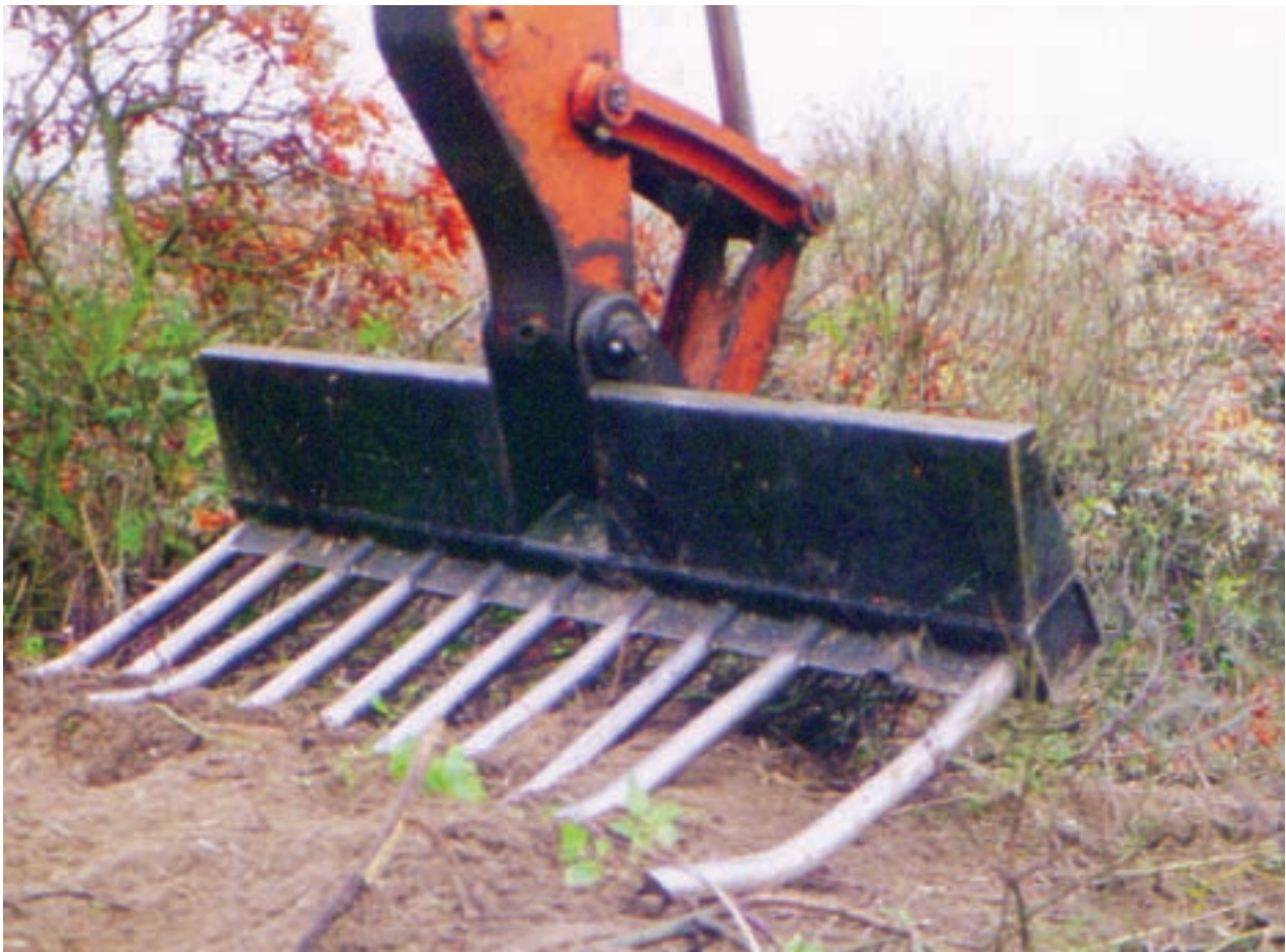
Plate 5 Close up of rake attachment on Hi-mac excavator.
